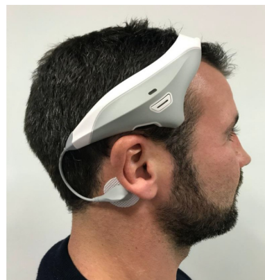
Figure 1: Battery-powered vestibular nerve stimulator (ML1000, Neurovalens, UK).
